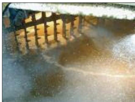
The malt is mashed to extract the sugars
