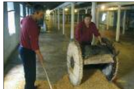
Laying the Barley on the malting floor after steeping
