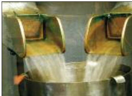
The clear spirit can be seen in the spirit safe
