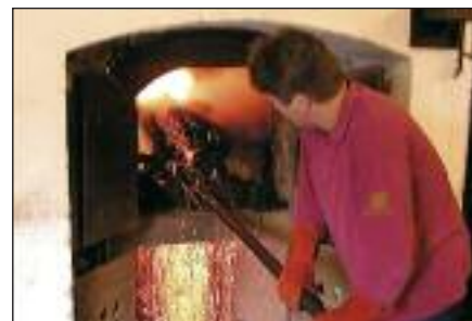
Stoking the kiln fire with peat and coke
