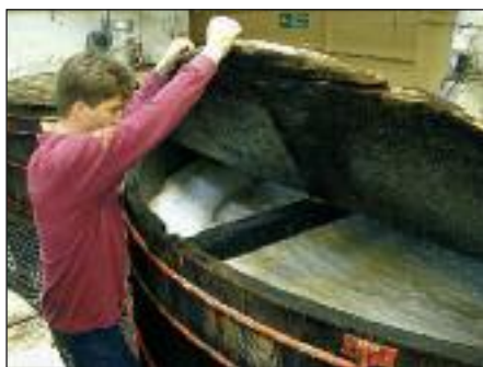
The mash is fermented in large wash backs
