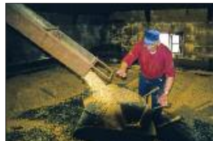
Loading the kiln with the malted barley
