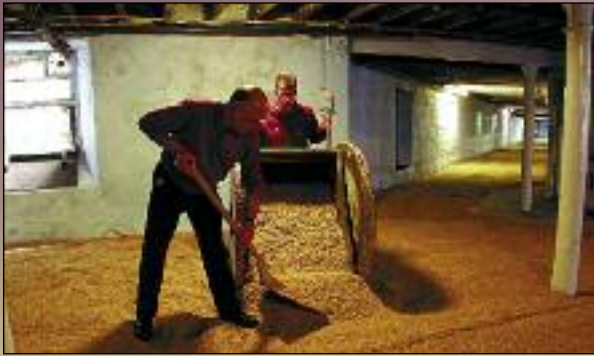
1 - Maltings - after steeping the barley, it is spread out on the malting floor and allowed to germinate
