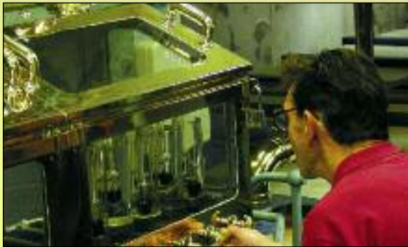
5 - Still Room - when fermentation is complete the result is distilled twice in the familiar pot stills.
