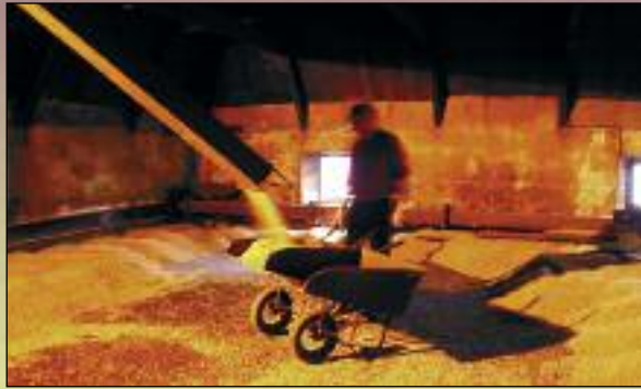
2- Loading the Kiln - the malted barley is then placed in the kiln where it is dried over a peat fire
